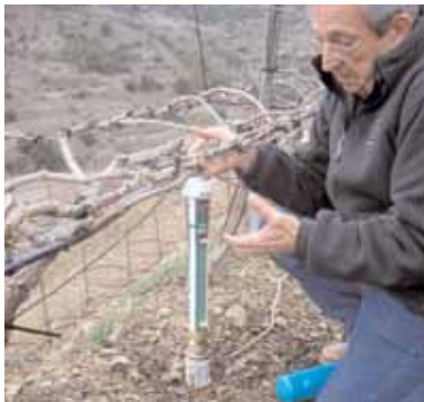
Sensors for measuring soil moisture at three depths: 35 cm, 50 cm and 70 cm
