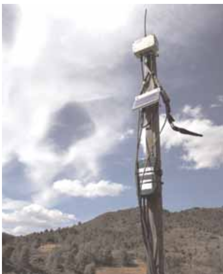
Data transmitter from the vineyard to the central office
